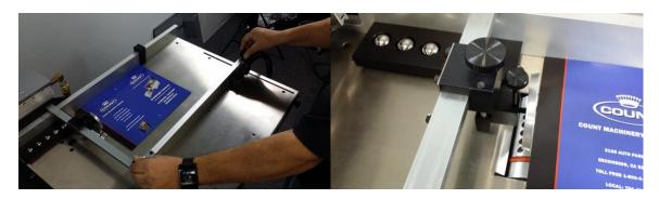
Loosen the lock knob on the back stop assembly and move it to the end of the sheet. DO NOT PINCH THE SHEET! This is to prevent the sheets from moving backward not to push the sheets forward. Loosen the front and rear lock knob on the operator side feed rail and adjust it up to the side of the paper. DO NOT PINCH THE SHEET! This is supposed to be aligned to the side of the sheet but not to pinch. Proper alignment of the rail is imperative to getting consistent feeding of stock.
