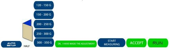
**TRI-FOLD SETUP:** Press the Auto Setup Button > Tri-Fold > Paper Thickness > Adjust the Knob Setting > OK, I have made the Adjustment > Start Measuring > Physically Run a sheet through the machine for the sensor to measure > Accept > Run.
