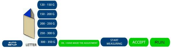
**GATE FOLD SETUP:** Press the Auto Setup Button > Tri-Fold > Paper Thickness > Adjust the Knob Setting > OK, I have made the Adjustment > Start Measuring > Physically Run a sheet through the machine for the sensor to measure > Accept > Run.
