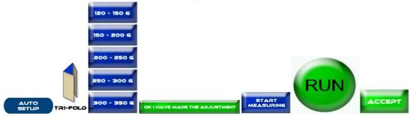
**Z FOLD SETUP:** Press the Auto Setup Button > Tri-Fold > Paper Thickness > Adjust the Knob Setting > OK, I have made the Adjustment > Start Measuring > Physically Run a sheet through the machine for the sensor to measure > Accept > Run.
