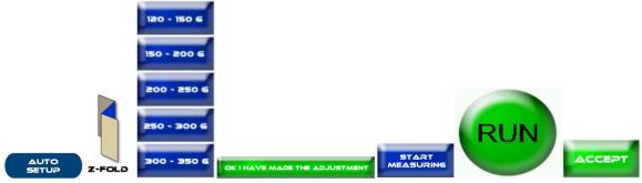
**LETTER FOLD SETUP:** Press the Auto Setup Button > Tri-Fold > Paper Thickness > Adjust the Knob Setting > OK, I have made the Adjustment > Start Measuring > Physically Run a sheet through the machine for the sensor to measure > Accept > Run.
