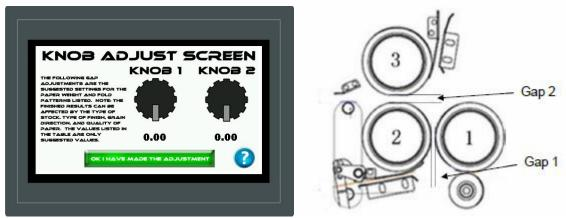
Make sure the setting is correct on the machine before pressing the OK, I HAVE MADE THE ADJUSTMENT Button.
