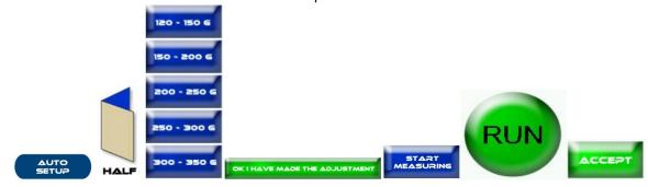
**TRI-FOLD SETUP:** Press the Auto Setup Button > Tri-Fold > Paper Thickness > Adjust the Knob Setting > OK, I have made the Adjustment > Start Measuring > Physically Run a sheet through the machine for the sensor to measure > Accept > Run.
