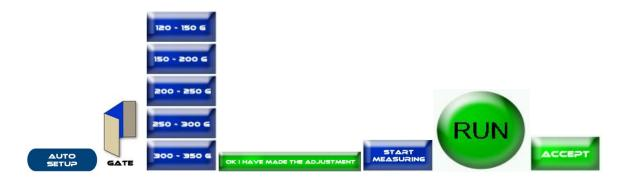
**DOUBLE PARALLEL FOLD SETUP:** Press the Auto Setup Button > Tri-Fold > Paper Thickness > Adjust the Knob Setting > OK, I have made the Adjustment > Start Measuring > Physically Run a sheet through the machine for the sensor to measure > Accept > Run.
