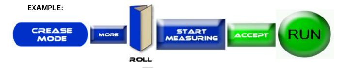
**Gate Fold:** Press the Crease Mode Button > More > Gate > Start Measuring > Physically Run a sheet through the machine for the sensor to measure > Accept > Run.
