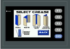
Crease selections include half, tri-fold, z fold, letter fold, roll fold, gate fold, double gate, double parallel, 3 perfect bind selections and 12 custom crease locations.
