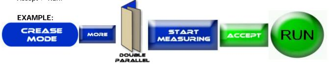
**Perfect Bind Double Hinge:** Press the Crease Mode Button > More > Perfect Binding Score > Enter The Book Thickness > Double Hinge > Start Measuring > Physically Run a sheet through the machine for the sensor to measure > Accept > Run.
