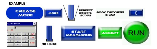
**Custom Crease Job:** Press the Crease Mode Button > Custom > Enter In Distance For each Crease in mm > Accept > Run.
