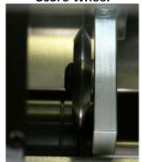
Position your score blade as desired. Scores should be made so that the blade runs on the side of the sheet that will be on the outside of the finished fold. Scores may be made on the EZ CREASER in three different ways using the different grooves on the lower score assembly.
