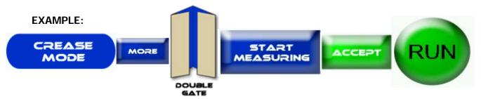
**Double Parallel Fold:** Press the Crease Mode Button > More > Double Parallel > Start Measuring > Physically Run a sheet through the machine for the sensor to measure > Accept > Run.
