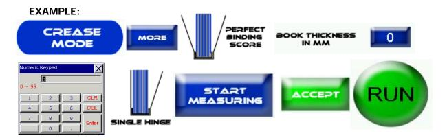
**Perfect Bind No Hinge:** Press the Crease Mode Button > More > Perfect Binding Score > Enter The Book Thickness > No Hinge > Start Measuring > Physically Run a sheet through the machine for the sensor to measure > Accept > Run.
