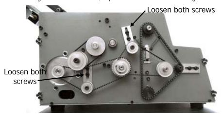
shaft should not be able to move side to side. With both drive belts in Position, re-tension the belt idlers and tighten while applying constant firm pressure on the belts by pushing down on the tops of the brackets with the large T-handle wrench supplied. Replace covers. Align upper assemblies accordingly.
