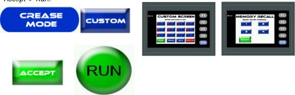
**Micro Adjusting the Crease Position:** Press the adjust button from the run screen. You can micro adjust each crease by pressing the arrow keys each direction. Each press will adjust by 1/13th of a mm. Each Adjustment is relative to the one before it so if you adjust crease 1 by 3 clicks it will also move all the creases after it. You would then need to adjust them back 3 clicks each.
