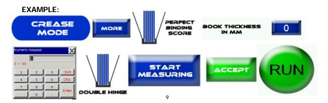
**Perfect Bind Single Hinge:** Press the Crease Mode Button > More > Perfect Binding Score > Enter The Book Thickness > Single Hinge > Start Measuring > Physically Run a sheet through the machine for the sensor to measure > Accept > Run.
