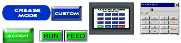
**Saving Custom Crease Jobs:** Press the Crease Mode Button > Custom > Enter In Distance For each Crease in mm > Save > Select Position to save in 1, 2, 3, or 4.
