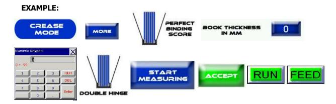
**Perfect Bind Single Hinge:** Press the Crease Mode Button > More > Perfect Binding Score > Enter The Book Thickness > Single Hinge > Start Measuring > Physically Run a sheet through the machine for the sensor to measure > Accept > Run > Feed.
