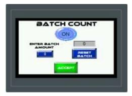
Press the Enter Batch Amount Button to enter in the number you want to run per batch.
