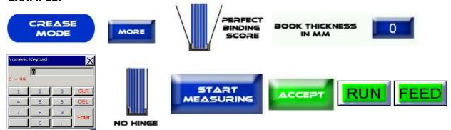
**Custom Crease Job:** Press the Crease Mode Button > Custom > Enter In Distance For each Crease in mm > Accept > Run > Feed.
