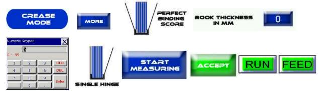
**Perfect Bind No Hinge:** Press the Crease Mode Button > More > Perfect Binding Score > Enter The Book Thickness > No Hinge > Start Measuring > Physically Run a sheet through the machine for the sensor to measure > Accept > Run > Feed.
