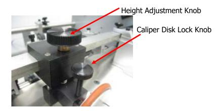
There are 2 different calipers; the o-ring and the metal caliper. The metal caliper is designed to work better with heavy stock and the o-ring caliper is designed to work with lighter stocks. Use the o-ring caliper when running any multi-part forms.
