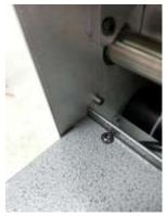
Install on top of the first dowel pin and under the second.
