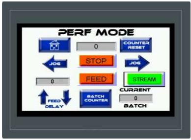
When the run button is pressed the graphic will change red and the button will flash. This is the indicator the machine is in running. When the feed button is pressed the graphics will change red and the paper will start to feed.
