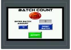
As you are running and the batch number is reached the screen will display "Batch Complete".
